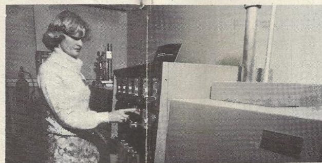
TO2 Fred Gigliotti tests micro-circuits in the Thick Film laboratory. Below Labs staffer Cheryl Crarey indicates the control panel of a bank of furnaces which fire thick film conductors at up to 850 deg C.
