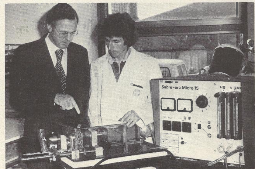
The Minister showed great interest in a sophisticated micro-welder which joins very thin metals. Showing him the technique is Senior Fitter and Turner Neil McKenzie.
