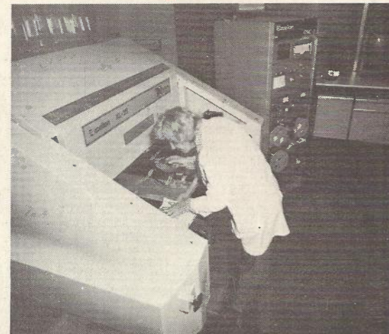
Tech. Asst. Eta Horvath setting up the Lab's new $ 70,000 numerically controlled machine which automatically and extremely accurately drills holes in printed circuit boards for exchanges. This was previously a very slow manual process giving varying quality.
