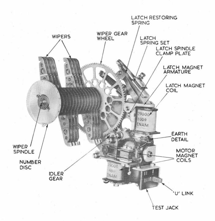
FIGURE 3. UNISELECTOR WIPER ASSEMBLY AND MOTOR.
