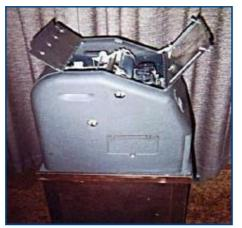
The case opens for access, as shown on this M15-RO.
