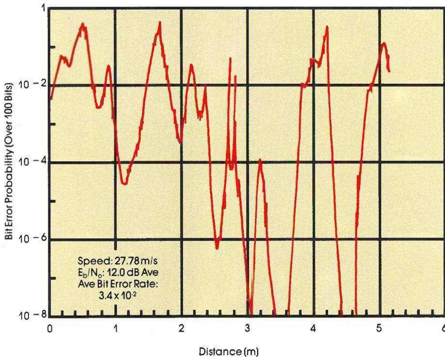
Variation of bit error probability over a 5m distance travelled by a mobile receiver in a typical urban mid-block location.
