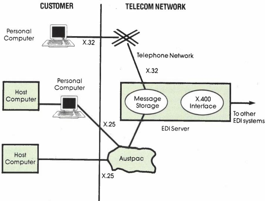
Schematic architecture of an EDI service based on OSI standards.
