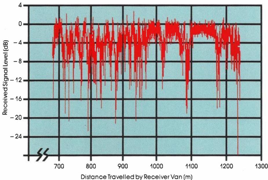
*Simulated mobile earth-to-space propagation results*
