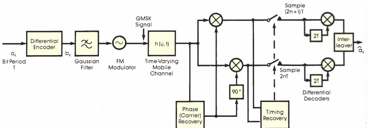
Schematic outline of a transmission system employing Gaussian Minimum Shift Keying (GMSK) modulation.
