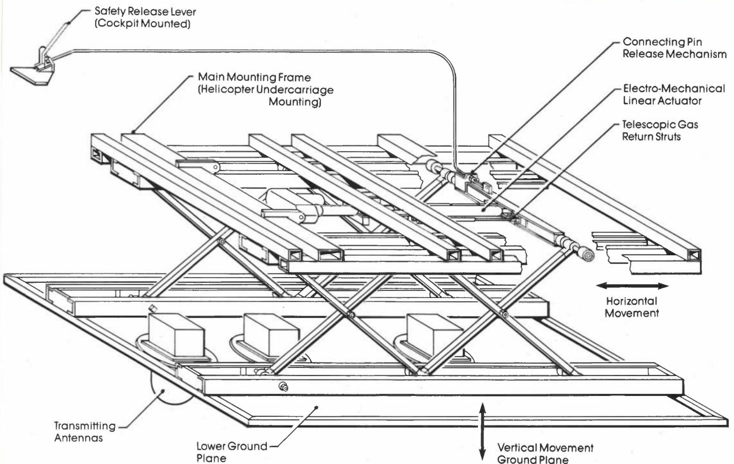
The Laboratories-designed helicopter antenna mount.
