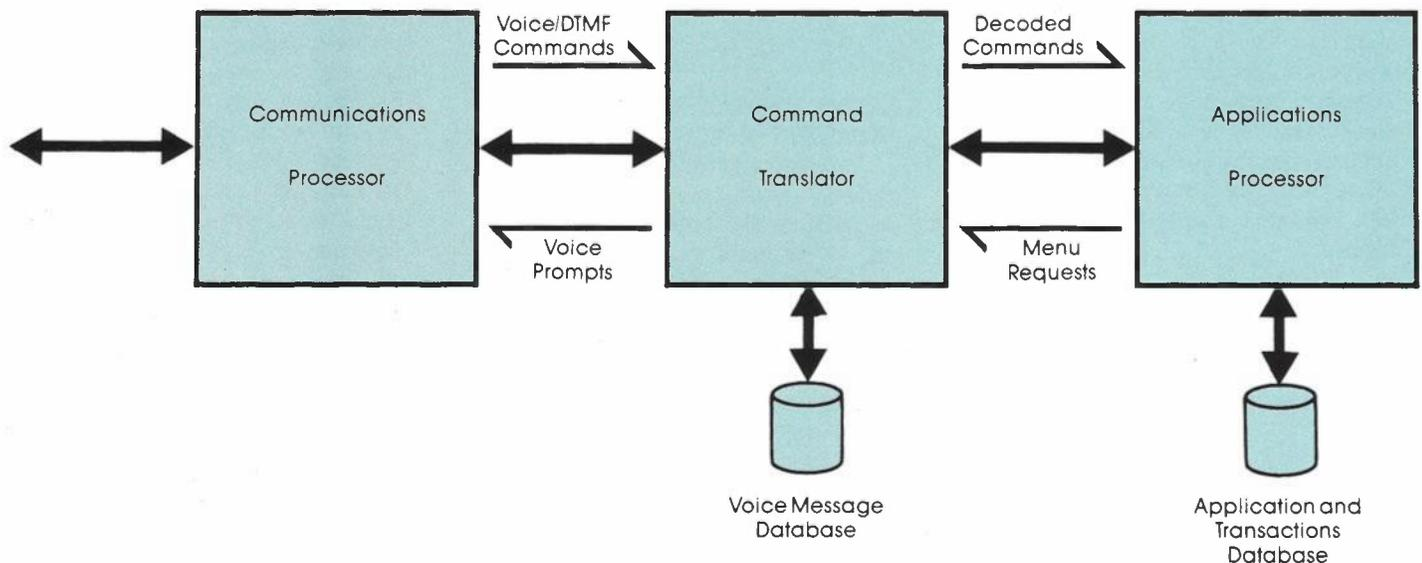
Detailed architecture of an intelligent peripheral providing voice value added services.
