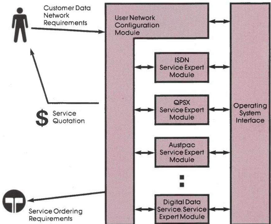
An integrated data network design tool for optimising specific customer services from Telecom's service options.
