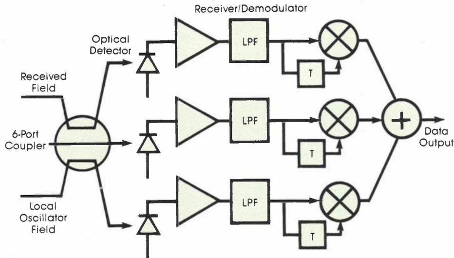
Schematic diagram of the optical phase-diversity receiver.
