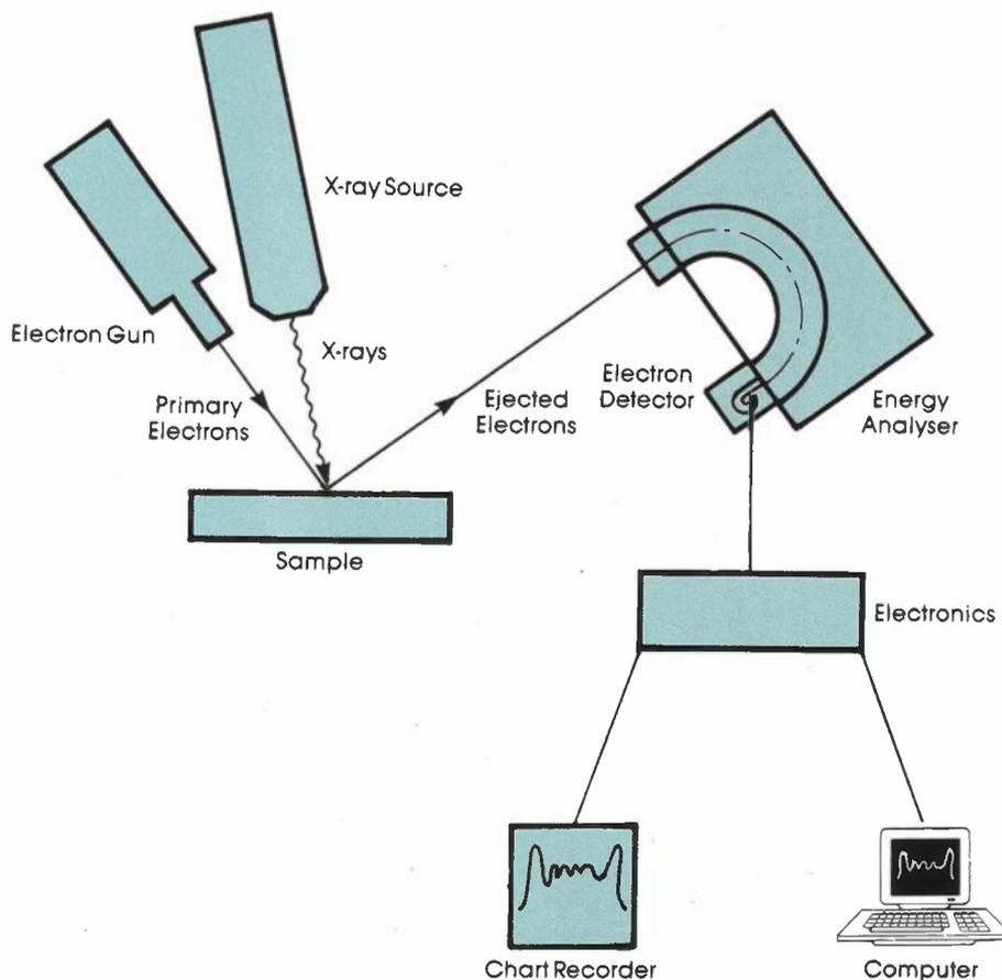
*Schematic representation of the components necessary for X-ray Photoelectron Spectroscopy and Scanning Auger Microanalysis.*
