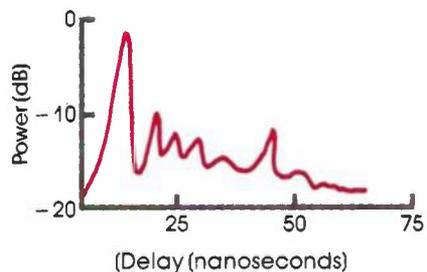
*Typical delay spread profile of a radio path in a wire-less office environment.*
