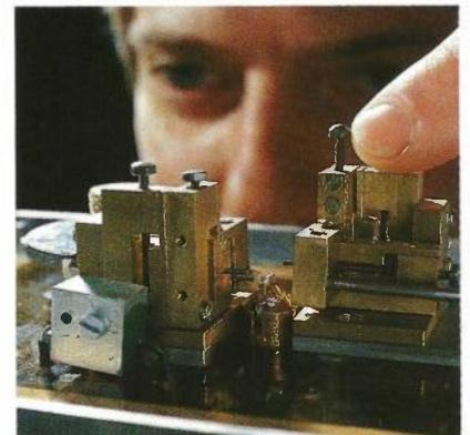
Linewidth reduction has been achieved in the laboratory by the use of an external cavity to introduce weak optical feedback to the laser diode. These external cavities consist of a short length of temperature controlled optical fibre with a mirrored endface. With this configuration, about a one thousand fold reduction of spectral linewidth has been achieved. Measurement of the narrow linewidth is performed using the delayed self-heterodyne technique.
