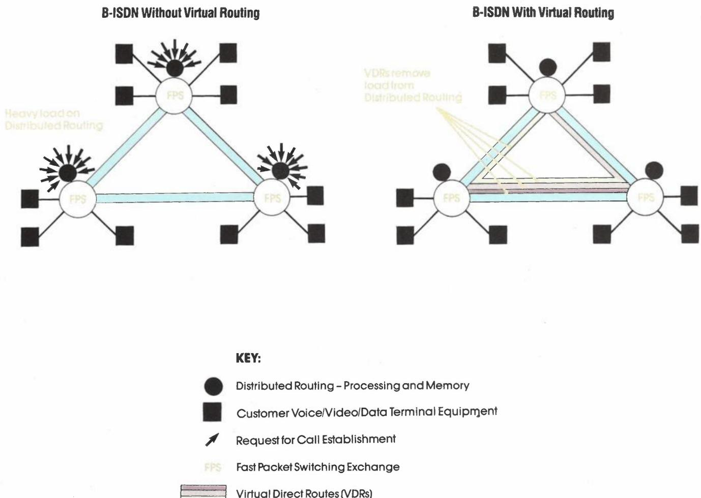
Virtual Routing reduces processing loads for resource allocation in the Broadband ISDN.
