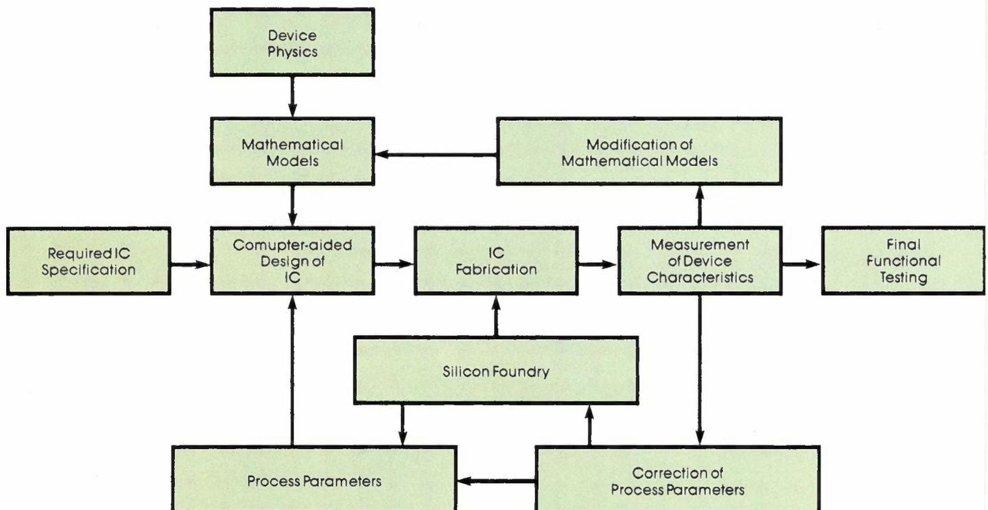
An illustration of the iterative process involved in the fabrication of integrated circuit devices.
