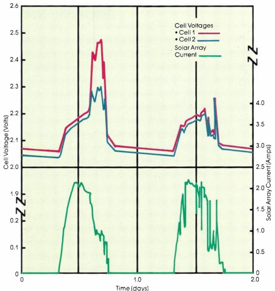
Solar power system parameters over a 2-day test period, showing potentials of two lead-acid cells versus solar array current.
