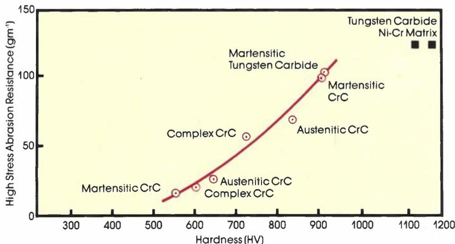
A plot of abrasion resistance for a series of hardfacing alloys. The terms austenitic and martensitic refer to matrix types, while the complex CrC type refers to the presence of additional alloying elements.
