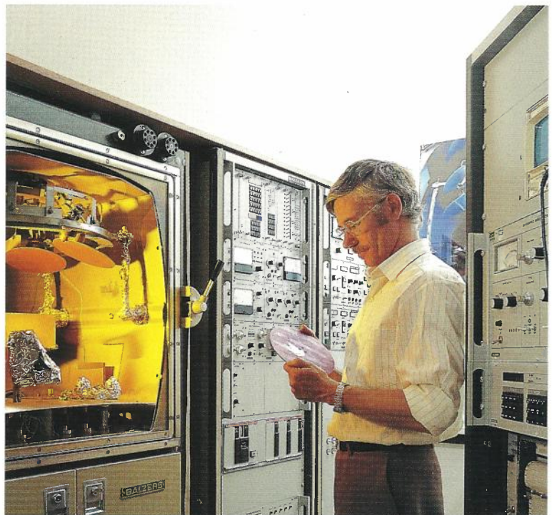
Gerry Brinson with TRL's Metal Evaporation System
