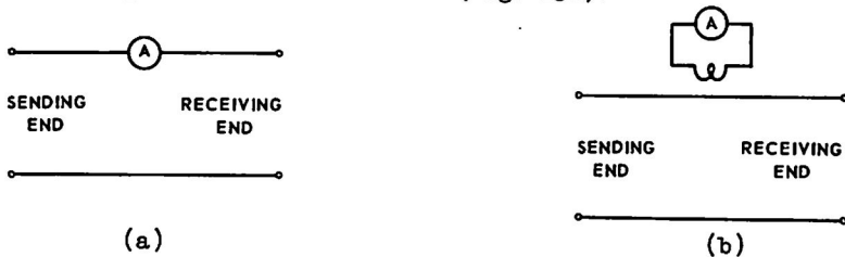
FIG. 23. MEASURING CURRENT ON OPEN WIRE LINES.
