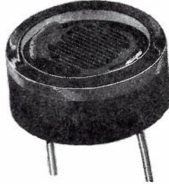
FIG. 17. TYPICAL LIGHT DEPENDENT RESISTOR (LDR).
