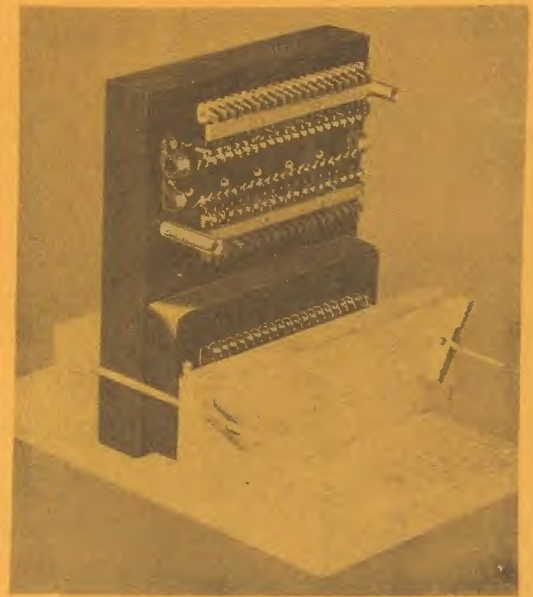
FIG. 4. JIG FOR FANNING OUT CABLES
