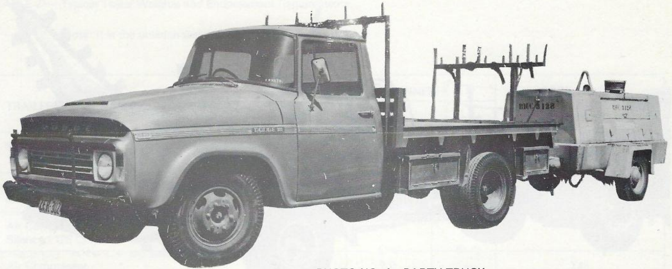
PHOTO NO. 4. PARTY TRUCK (TARE LESS THAN 3t) TOWING 250 CFM COMPRESSOR (TARE GREATER THAN .75t)
