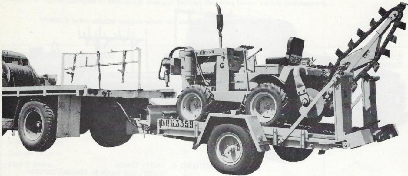
PHOTO NO. 6. WINCH TRUCK (TARE GREATER THAN 3t) TOWING V-30 ON TRAILER (TARE GREATER THAN 0.75t)
