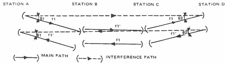
Note: The ratio (wanted signal/interfering signal) depends on the gain of the antennae at angles  $\phi_1$  and  $\phi_2$  relative to the gain in beam and the difference of propagation losses between main and overreach paths.
