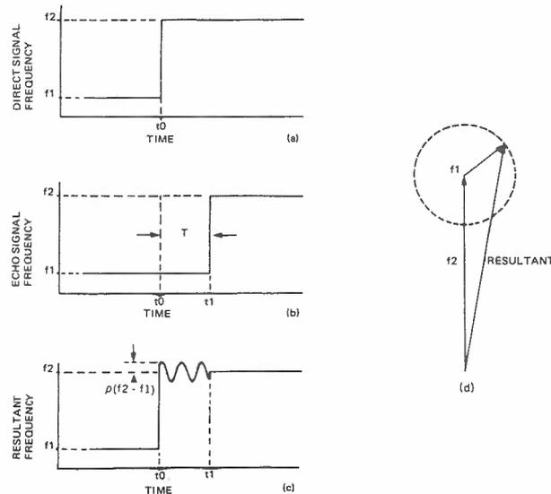
FIG. 21. EFFECT OF ECHO ON TELEVISION SIGNALS
