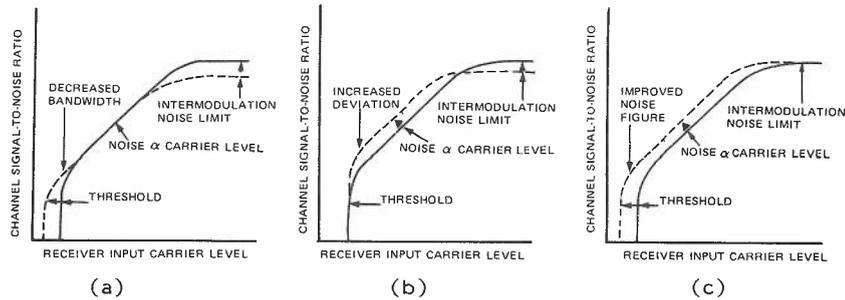
FIG. 23. FACTORS AFFECTING SIGNAL-TO-NOISE RATIO CHARACTERISTICS
