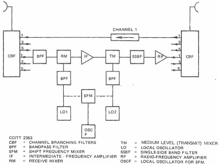
Note: The block marked channel 1 is a replica of the repeater shown in more detail for the opposite direction of transmission. Channels 3 and 5 will comprise similar repeaters operating on different radio frequencies.
