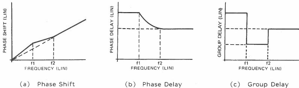
FIG. 7. COMPARISON OF PHASE SHIFT, PHASE DELAY AND GROUP DELAY
