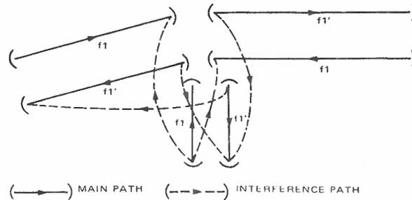
FIG. 35. SPUR ROUTE INTERFERENCE
