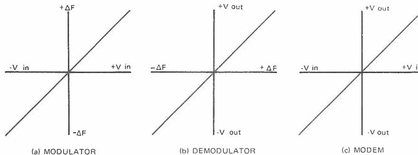
FIG. 15. FREQUENCY MODEM CHARACTERISTICS
