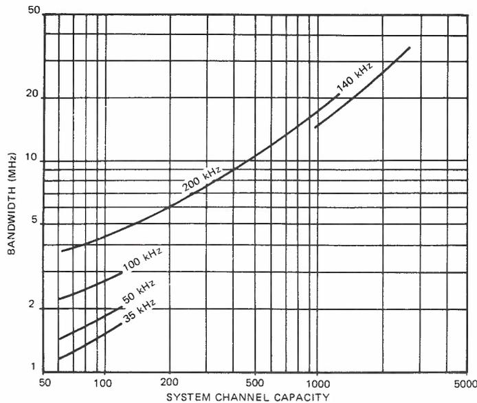
FIG. 4. BANDWIDTH REQUIREMENTS OF FM TELEPHONY BEARERS
