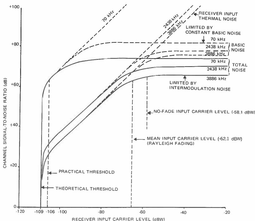
FIG. 25. SIGNAL-TO-NOISE RATIO FOR BASEBAND CHANNELS
