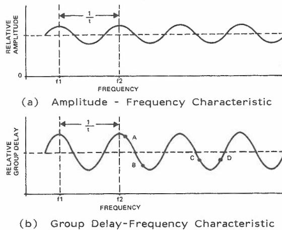
FIG. 19. EFFECT OF ECHOES ON AMPLITUDE-FREQUENCY AND GROUP DELAY - FREQUENCY CHARACTERISTICS
