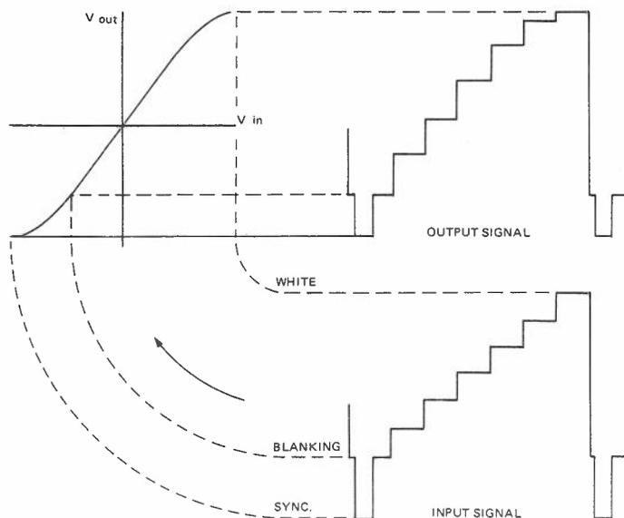
FIG. 13. EFFECT OF NON-LINEAR SYSTEM ON MONOCHROME TELEVISION SIGNAL
