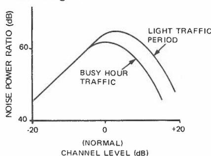
FIG. 32. EFFECT OF TRAFFIC DENSITY ON SIGNAL-TO-NOISE RATIO
