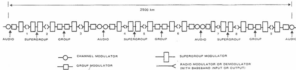
FIG. 37. CCIR HYPOTHETICAL REFERENCE CIRCUIT (RADIO BROADBAND TELEPHONY BEARER)
