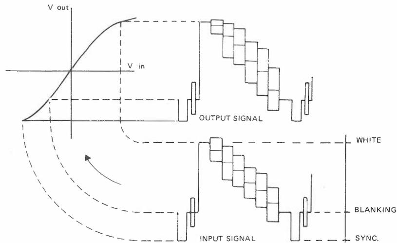
FIG. 14. EFFECT OF NON-LINEAR SYSTEM ON COLOUR TELEVISION SIGNAL
