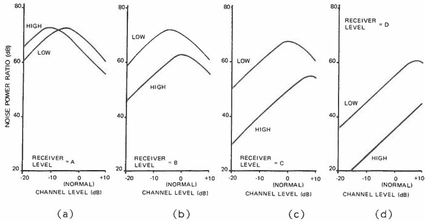
FIG. 31. SIGNAL TO NOISE RATIO-CHANNEL SIGNAL LEVEL CHARACTERISTIC
