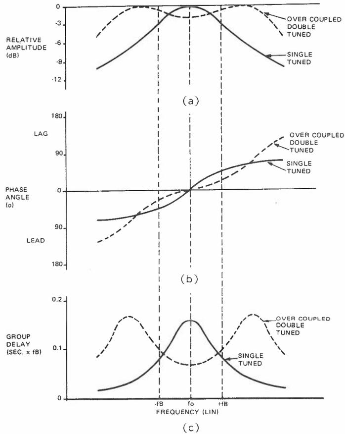
FIG. 8. CHARACTERISTICS OF TUNED AMPLIFIER
