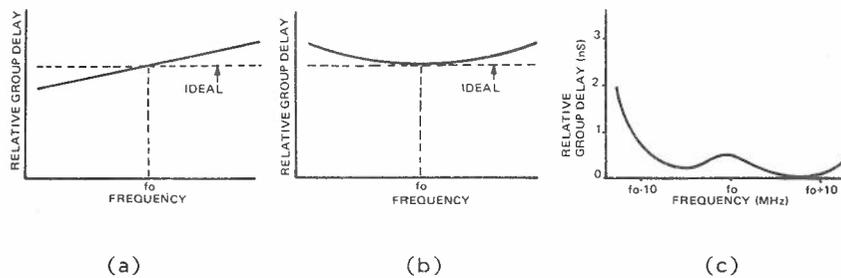
FIG. 18. GROUP DELAY CHARACTERISTICS
