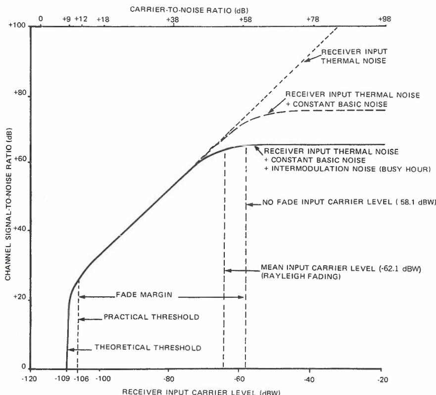
FIG. 22. VARIATION OF SIGNAL-TO-NOISE RATIO WITH CARRIER LEVEL
