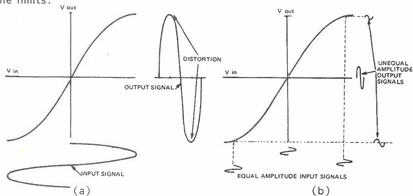
FIG. 1. EFFECTS OF AMPLITUDE NON-LINEARITY
