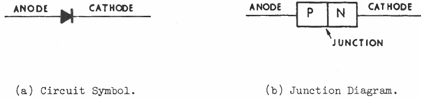
FIG. 3. SEMICONDUCTOR JUNCTION DIODE.
