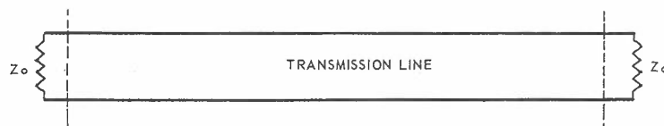
FIG. 38. TERMINATING THE INPUT AND OUTPUT OF A LINE IN ITS CHARACTERISTIC IMPEDANCE.
