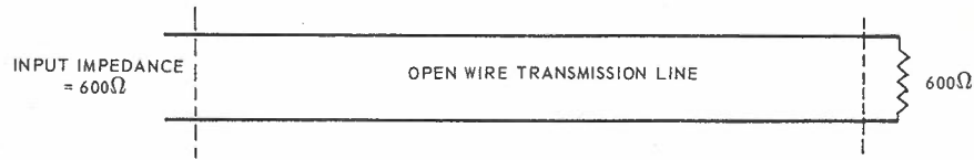
FIG. 35. TERMINATING A LINE IN IT'S CHARACTERISTIC IMPEDANCE.
