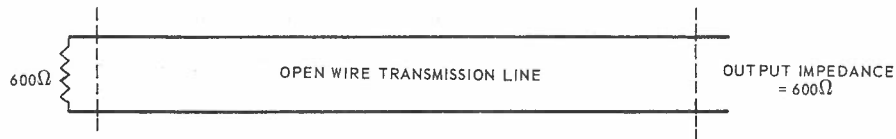
FIG. 37. TERMINATING THE INPUT OF A LINE IN ITS CHARACTERISTIC IMPEDANCE.
