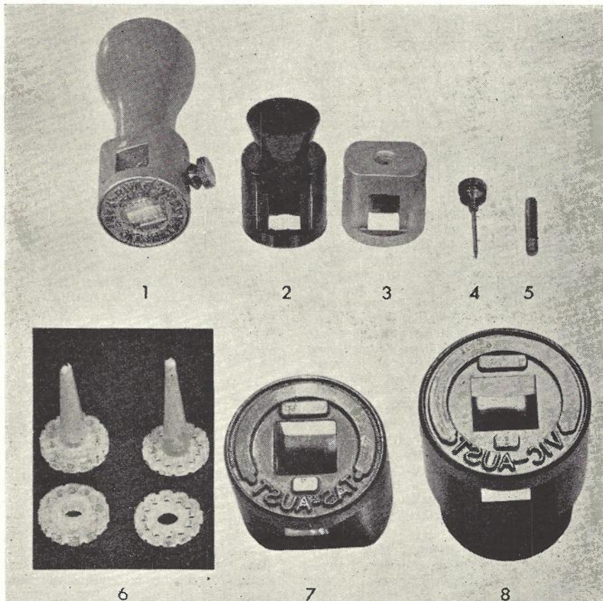
1. Complete Postmarker for 1957 Antarctic Expedition. 2. Polystyrene Pattern for Investment Casting of Body. 3. Investment Cast Nickel Steel Body. 4. Locking Pin. 5. Number Wheel Shaft. 6. "Nylon" Number Wheels, Before, After Trimming Sprue. 7. Details of Engraving as Normally Investment Cast. 8. Polystyrene Pattern.
