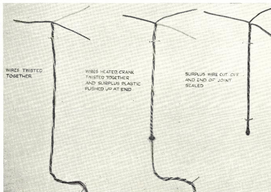
Fig. 1 — Multiple Joint made by Hot Twist Method.
