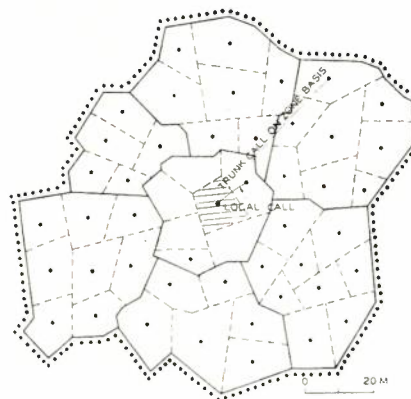
TRUNK CHARGING ON ZONE BASIS.
