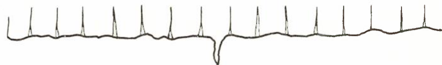
Fig. 7 — Trace Showing Short-circuit Fault, 37.5 Miles from Testing Station, on Same Circuit as Fig. 5.
