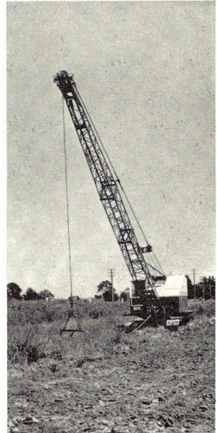
Fig. 6.—22RB Excavator rigged as Dragline.
