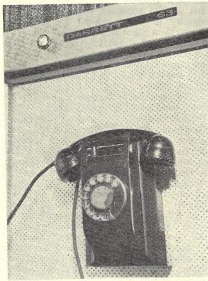
Fig. 1.—Telephone Booth Visual Indicator.
