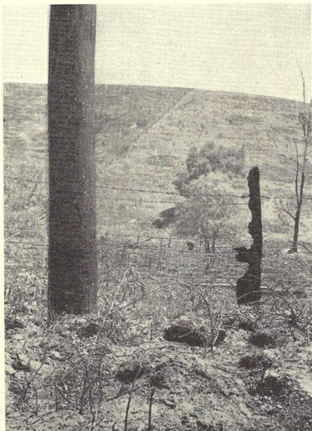
Treated pole alongside burnt out fence. Note blackberry canes which show that pole was surrounded by growth.
