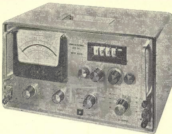
M.T.S. A210—Audio/Ultrasonic Test Set for the complete evaluation of audio and ultrasonic amplifiers, filters and transmission circuits.
