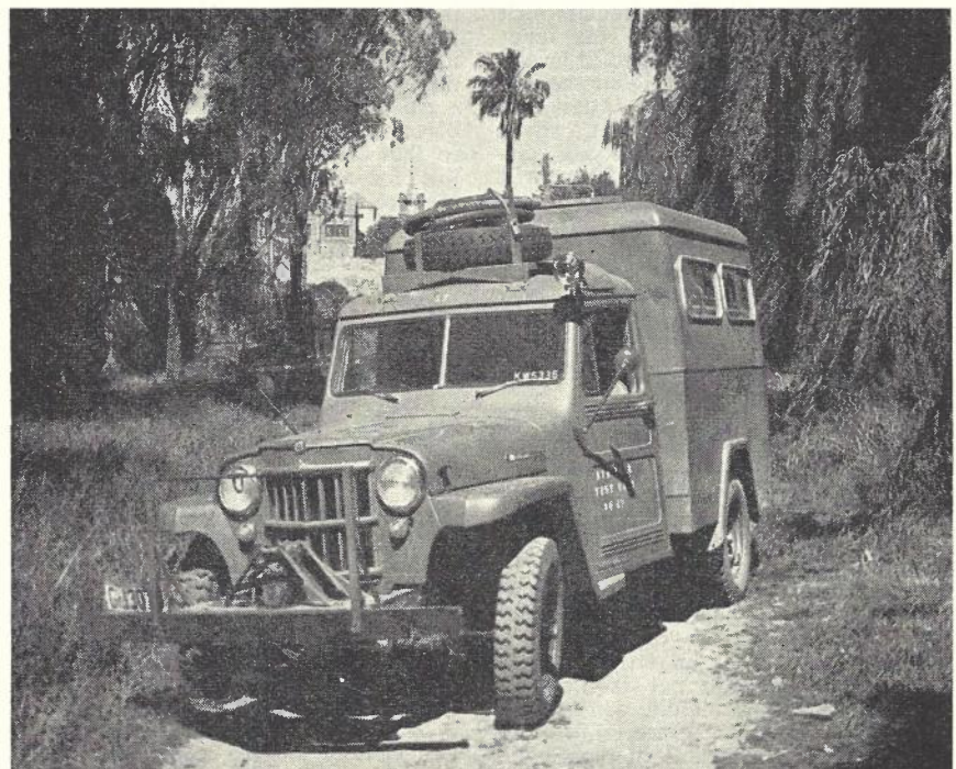
Fig. 5.—Typical Country Patrol Vehicle with Front Mounted Sludge Pump.
