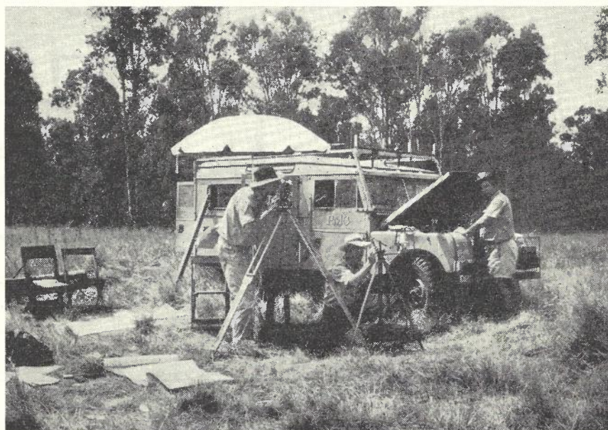
Fig. 1.—Field Party Surveying on Brisbane-Cairns Route. The party is using an accurate (1 second) theodolite, heliograph, and 80 watt spotlight.
