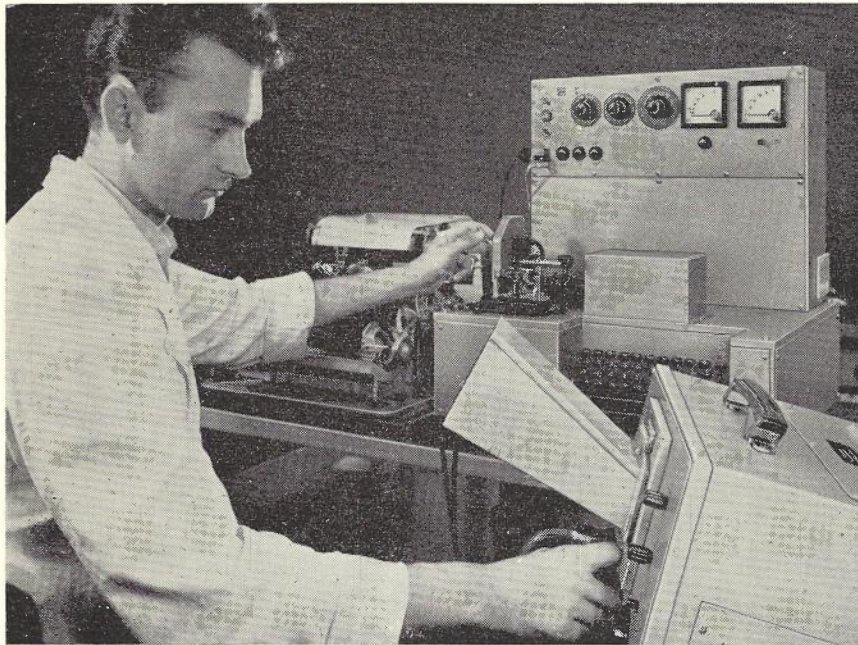
Fig. 8.—Test Bench for Adjusting Transmitter to Minimum Distortion.
