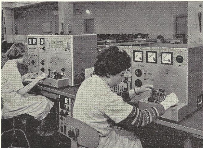
Fig. 10.—Test Benches for the Electrical Test of one Receiver. Receive margin and tripping delay, among other functions, are tested here.
