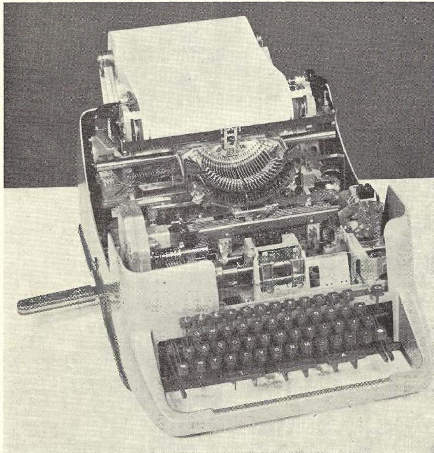
Fig. 5.—Printer Base and Type Basket. Both test pieces have been assembled into a printer and placed in a test fixture (with keyboard). The lever (left) is used for easy clamping and releasing of test pieces.
