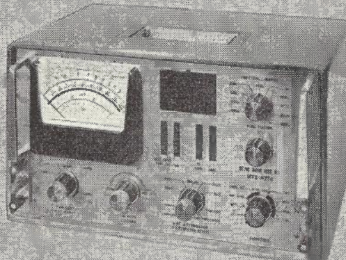
M.T.S. A310—MF/HF Radio Equipment Test Set for checking medium-frequency and high-frequency radio communication equipment, particularly marine installations.
