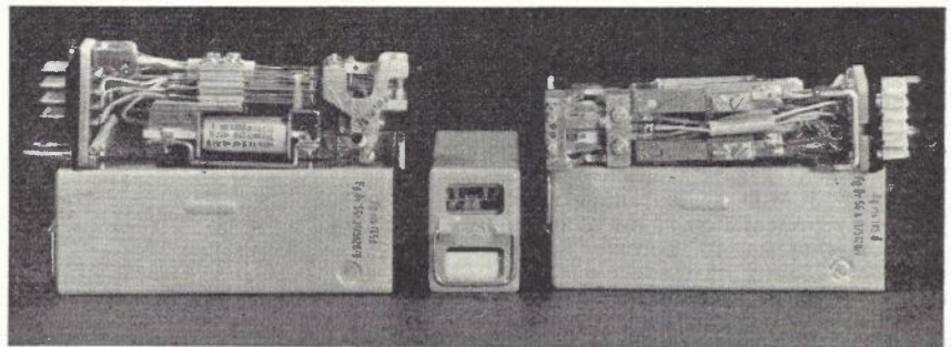
Fig. 7 — High Speed Relays.
