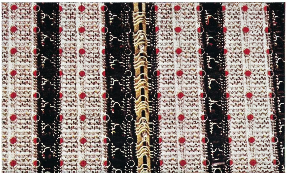
(BOTTOM RIGHT) Frame assembly illustrating the wiring gutters used to accommodate the tape wiring.
