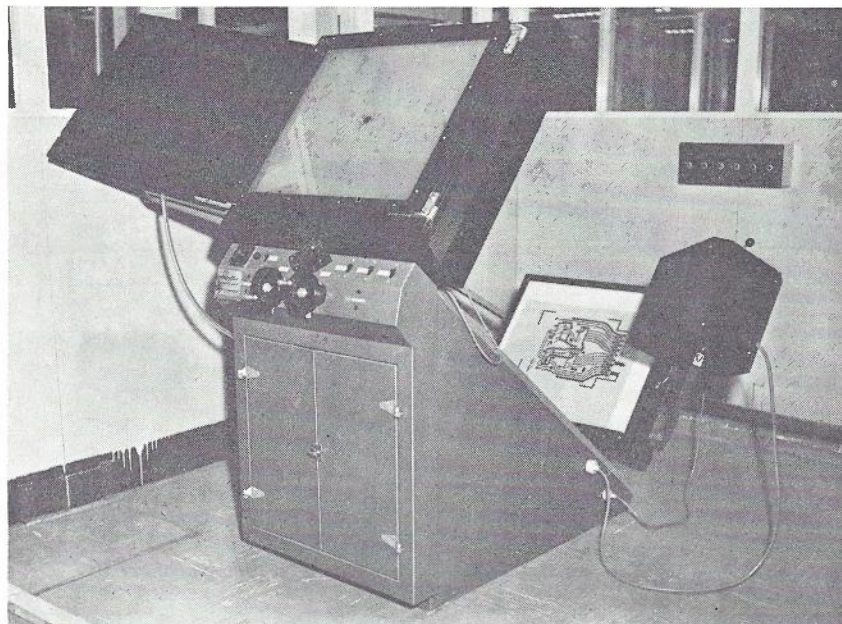
Fig. 4 — A Typical Process Camera Suitable for Photo-Reduction of Printed Wiring Artwork.
