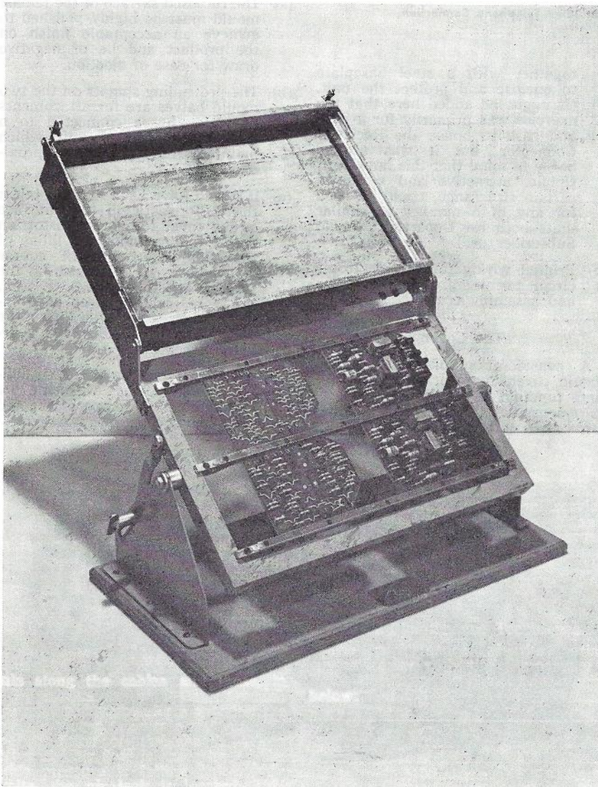
Fig. 17 — Assembly Jig for Circuit Boards.
