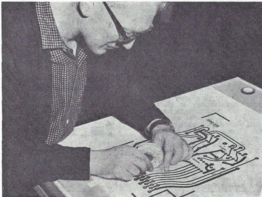
Fig. 3 — Laying down Taped Conductor Paths from a Tape Dispenser.
