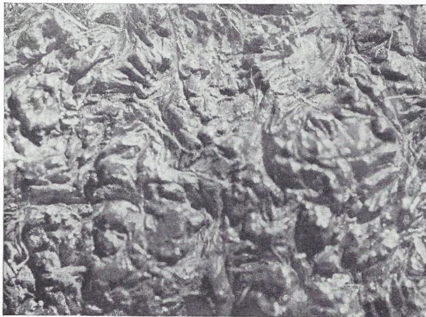
Fig. 6 — Termite Mandible Markings on Lead Sheath.
