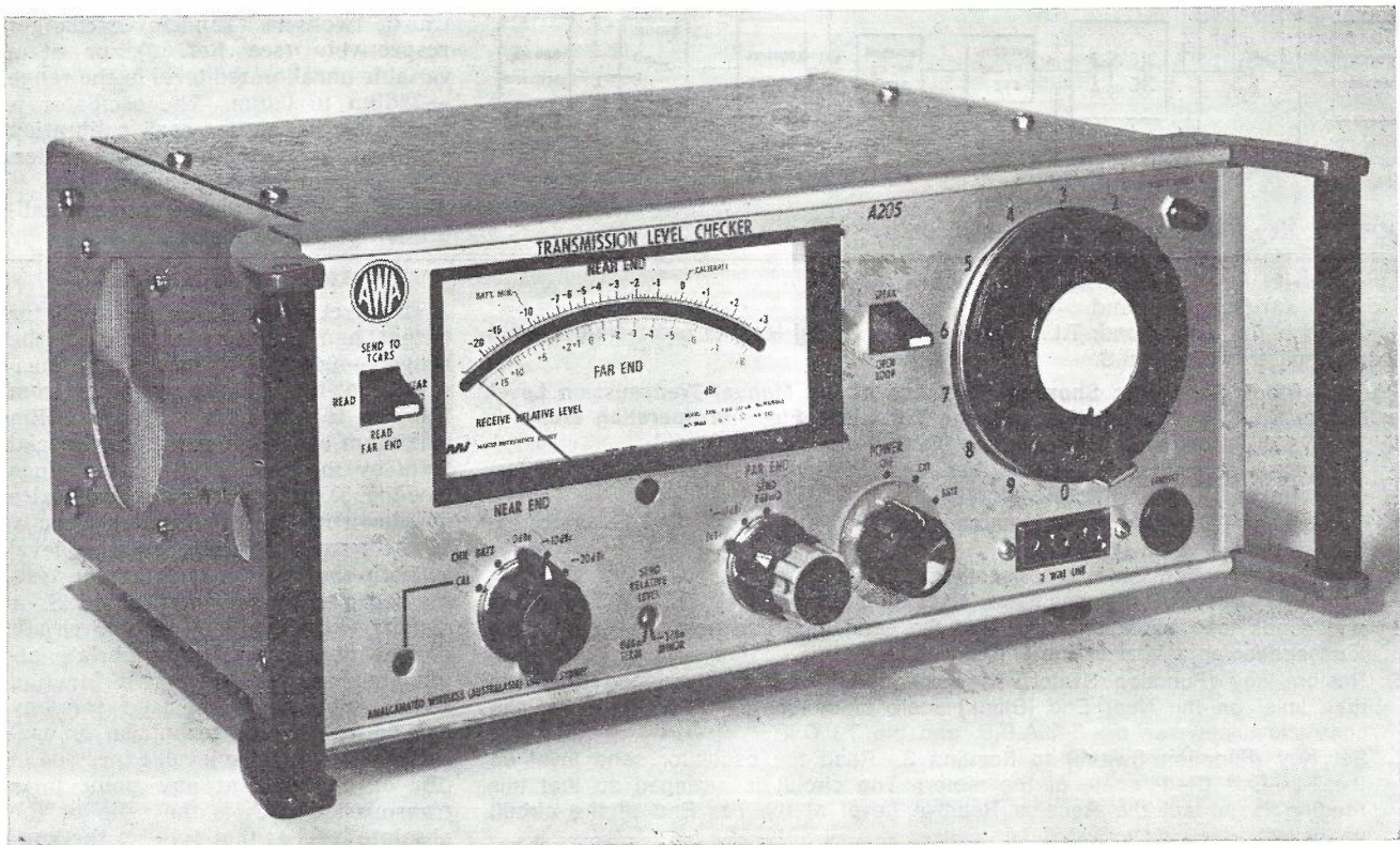
Fig. 1 — The Transmission Level Checker Type A205. The speaker grill and slot for screwdriver speaker volume adjustment can be seen on left hand side panel.
