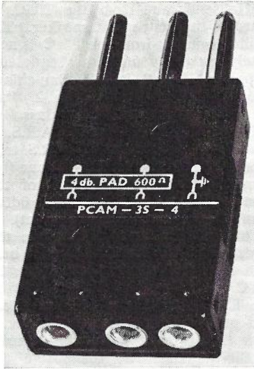
Fig. 3 — The 4dB Attenuator Pad. It is used to extend the range of the T.L.C. and is plugged into the T.L.C. and the measuring cord plugged into the back of the pad. Note 4MM connector.
