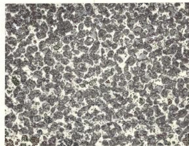
Fig. 4.—Photomicrograph showing structure of 30-70 Tin-Lead Solder.
