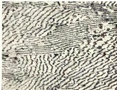
Fig. 2.—Photomicrograph showing structure of eutectic Tin-Lead Solder.
