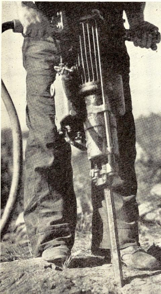
Fig. 2.—“Barco” Hammer in operation. The hose at left carries leads to coil and battery.
