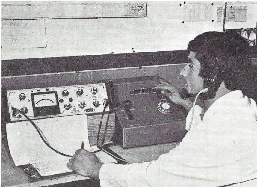
Fig. 2. — Interim Test Position in Use at the Geelong ARM Exchange.
