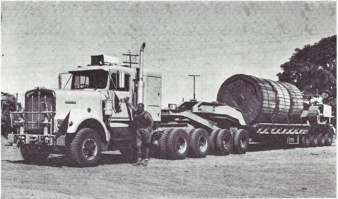
Fig. 11. — A Kenworth 50 ton Low Loader. On the rear is a tracked cable drum trailer capable of handling the 5 ton, 7ft. x 5ft., coaxial cable drums.
