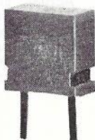
MODEL BFB-455A improves the selectivity of transistor radios when used as an emitter by-pass in transistor IF Stages.
