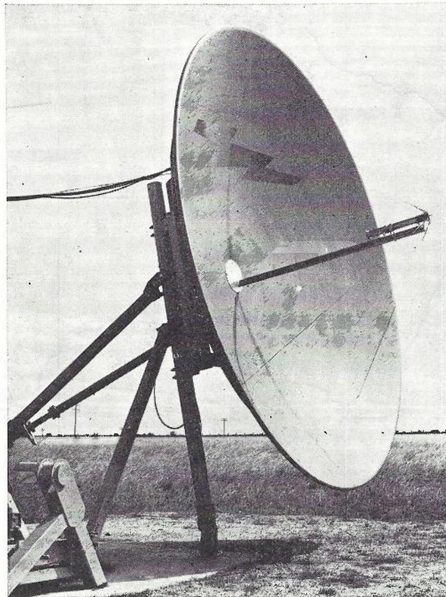
Fig. 3 — Outstation Antenna for Subscriber's Equipment Experiment.
