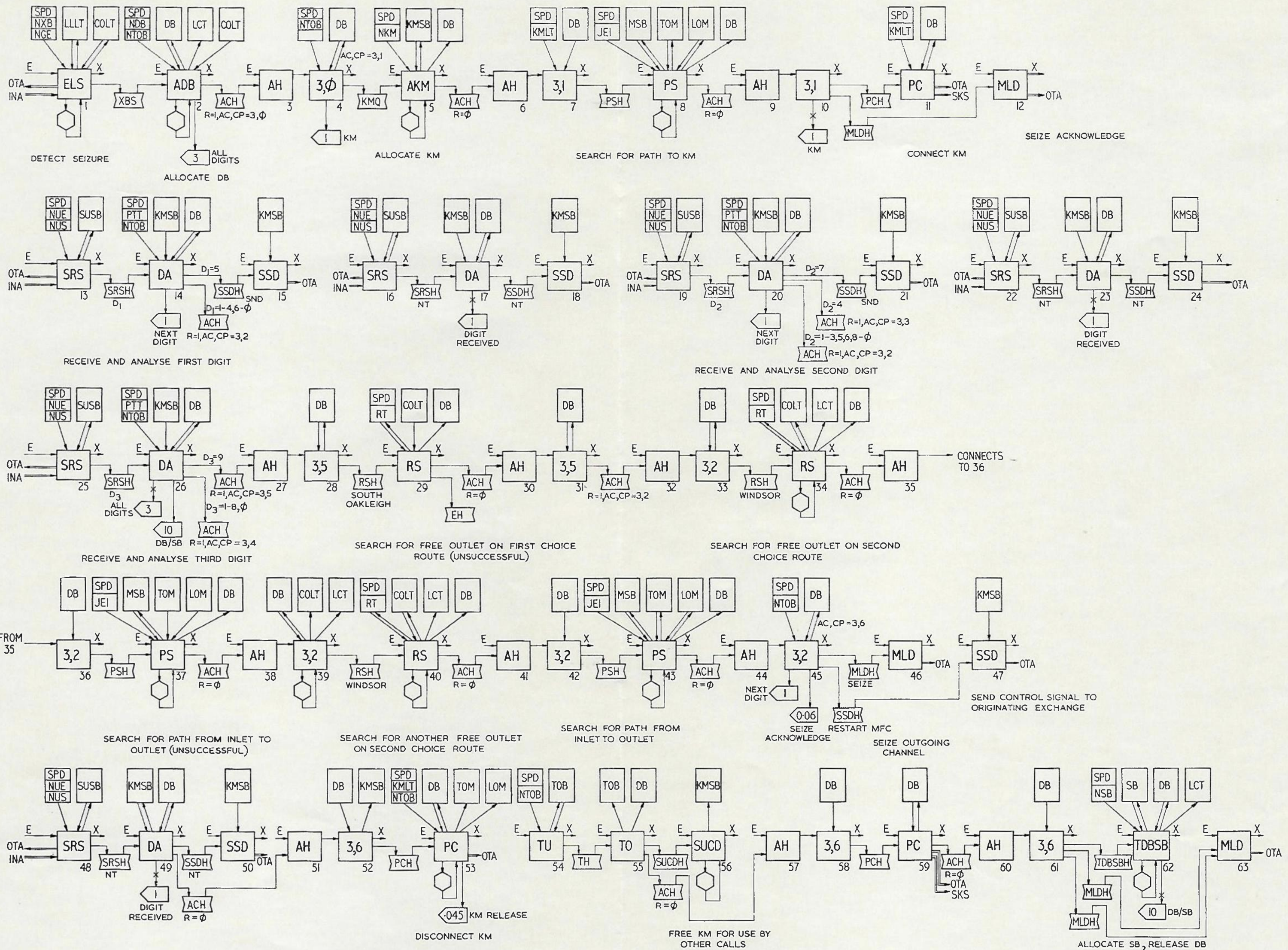
Fig. 26 — Program Sequence for a Simple Successful Call from Clayton to South Oakleigh
