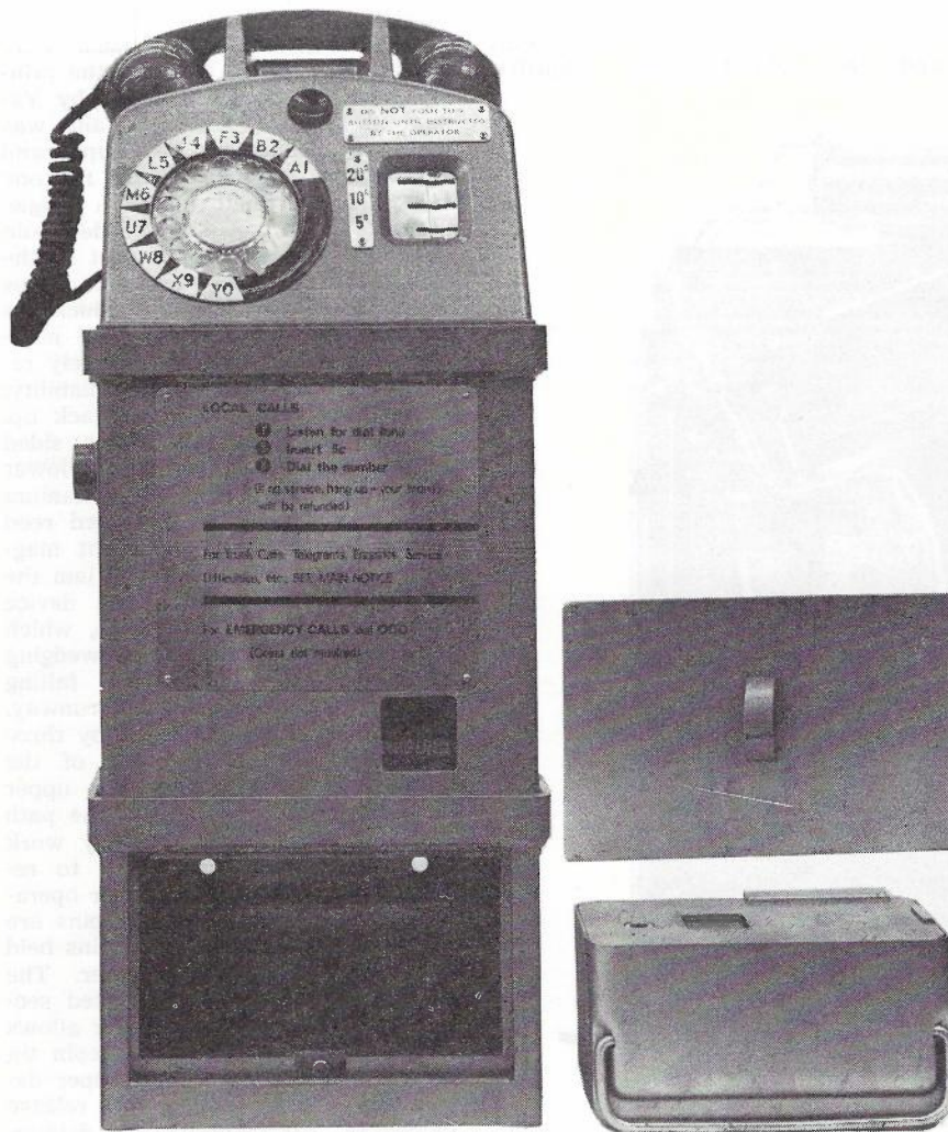
Fig. 6. — Strengthened Coin Telephone No. 1 Case, Showing Coin Safe Door Arrangement.
