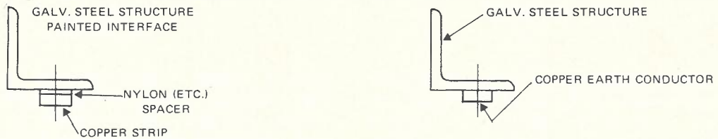
FIG. 18 MOUNTING LIGHTNING CONDUCTOR
