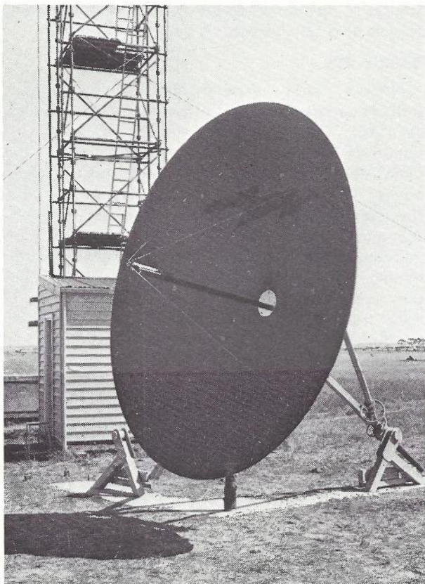
Fig. 2—This Antenna is Typical of those which might be used for Providing Communications to Remote Areas via an Australian National Satellite. It is about 4 metres in diameter and uses a relatively simple mount which allows it to be manually aligned with the satellite. In 1969-1970, it was used in an APO demonstration experiment with the ATS-1.
