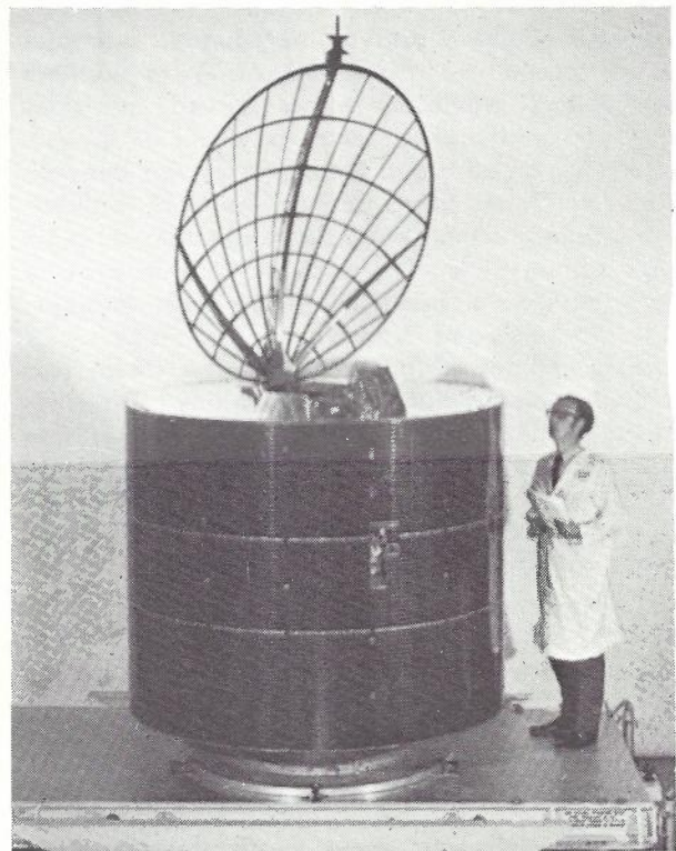
Fig. 5—The Canadian ANIK Spacecraft. Two have been launched, in November, 1972 and April, 1973, and a third is scheduled for launch in 1975. The body, covered with solar cells, rotates to provide gyroscopic stabilization, while the antenna on top of the satellite stays pointed at earth. (Photo courtesy of Hughes Aircraft Company).
