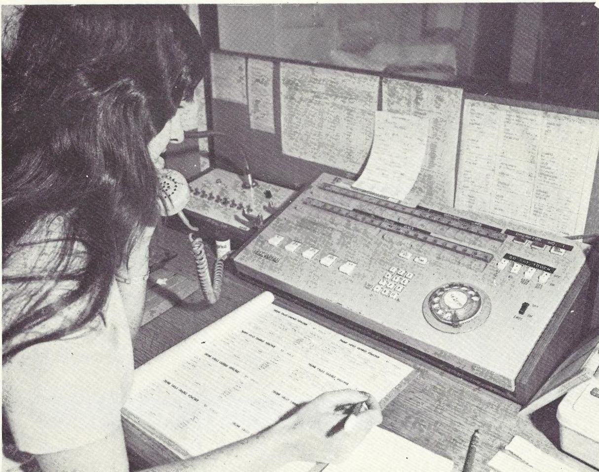
Fig. 11—Operators Console Hitachi AX2X PABX, Hotel Melbourne.
