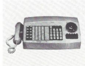
PABX—manufactured by Plessey Australia, Telecommunications Division, this private automatic branch exchange system employs crossbar switching and componentry similar to that used by the Australian Telecommunications Commission in the national telephone network.
