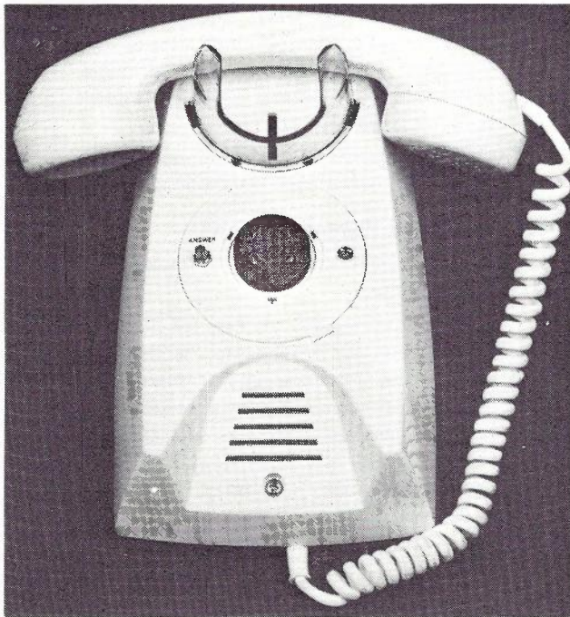
Fig. 2 — Bearer Surveillance Status Equipment at long line equipment control stations. The facilities have been built into the telephone. The status monitoring facility is disconnected whilst the telephone is in use as an order wire to the SRTC centre.
