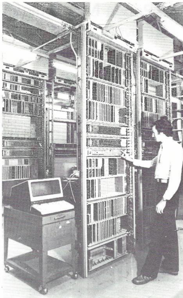
Fig. 5 — General View of the ARE-11 Delivery Testing Equipment at the Broadmeadows Plant of L M Ericsson. The test positions for the testing of equipped shelves are at a height suitable for easy access and handling during the test.
