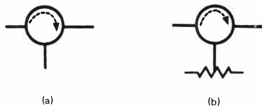
Fig.10-Circulator and Isolator Symbols
