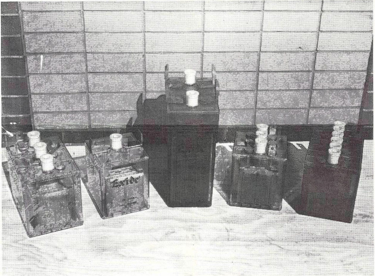
Fig. 32 — Telecom Pasted-Plate Lead-Acid Batteries from L to R: 6V — 90 Ah, 2V — 200 Ah, 2V — 500 Ah, 6V — 45 Ah, 12V — 25 Ah.
