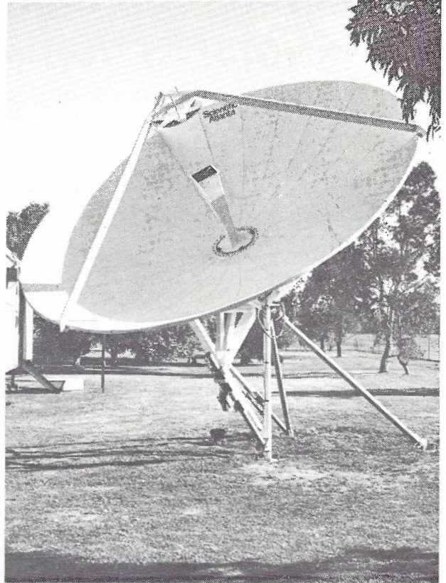
The small satellite earth station which was recently used to test the feasibility of providing the television to remote areas of Australia using the Pacific Intelsat satellite. The station was leased from Plessey Australia for the test.
