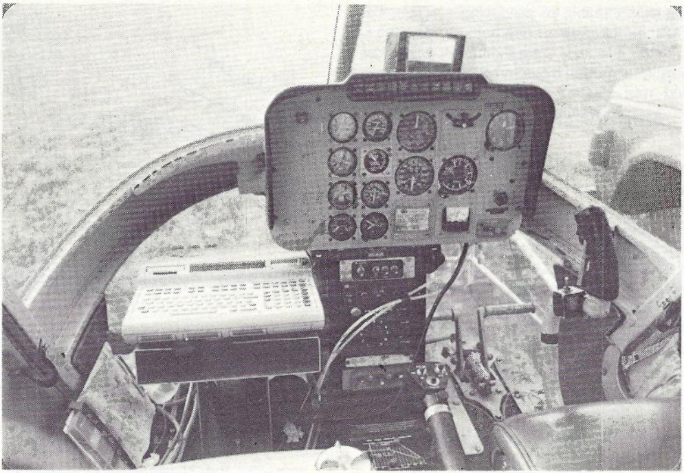
Fig. 11 — Radar Profiler Helicopter Installation
