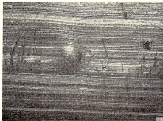
Fig. 3A.—Manufacturing defect. Photomicrograph × 8 diameters showing a transverse crack close to a "dross" protruberance on the sheath.
