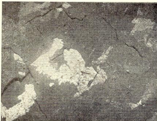
Fig. 1.—Inter-crystalline fracture of Cable Sheath. Etched section showing cracks following crystal boundaries.
