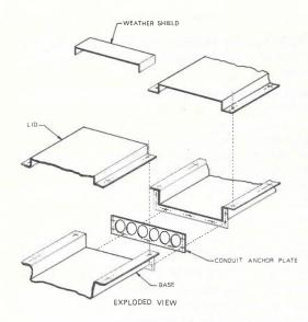
Fig. 7 — The Box Section Beam with the Conduit Anchor Plate.
