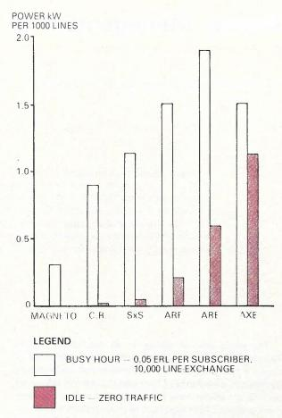
Fig. 2 — Power Requirements for Switching Systems.
