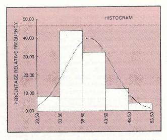
Fig. 3 — Histogram with Superimposed Normal Curve for Chi-Squared Test
