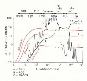
Fig. 1 — Attenuation Due to Atmospheric Constituents
