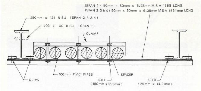
Fig. 2 — The PVC Support Bracket with the Clamp in Position.
