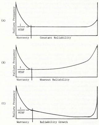
The above failure rate curves show how three different kinds of reliability in telecommunications equipment will vary throughout their lives. Several years ago one of the authors of this article introduced Reliability Growth and reduced Maintenance Cost to Telecom Australia equipment by failed component analysis and improved component reliability in replacement components.
