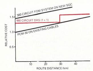
Fig. 3 — Average Cost of Provision of Switched Telephone Circuits in Metropolitan Areas Assuming ARF Exchanges
