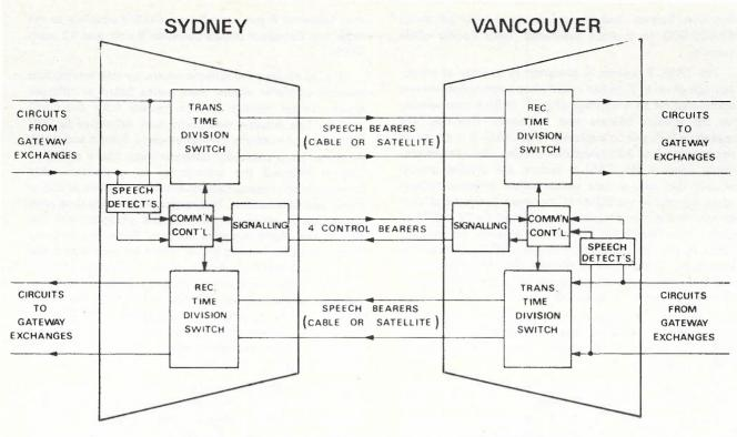
Fig. 2 - Simplified Block Diagram of the TASI-B system
