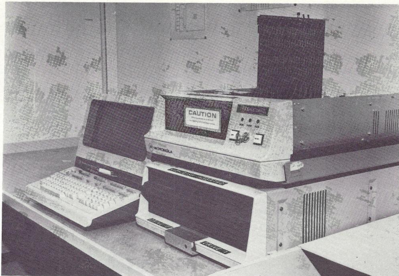
Fig. 4. Motorola EXORciser with EXOR Disc and Hewlett Packard Terminal.
