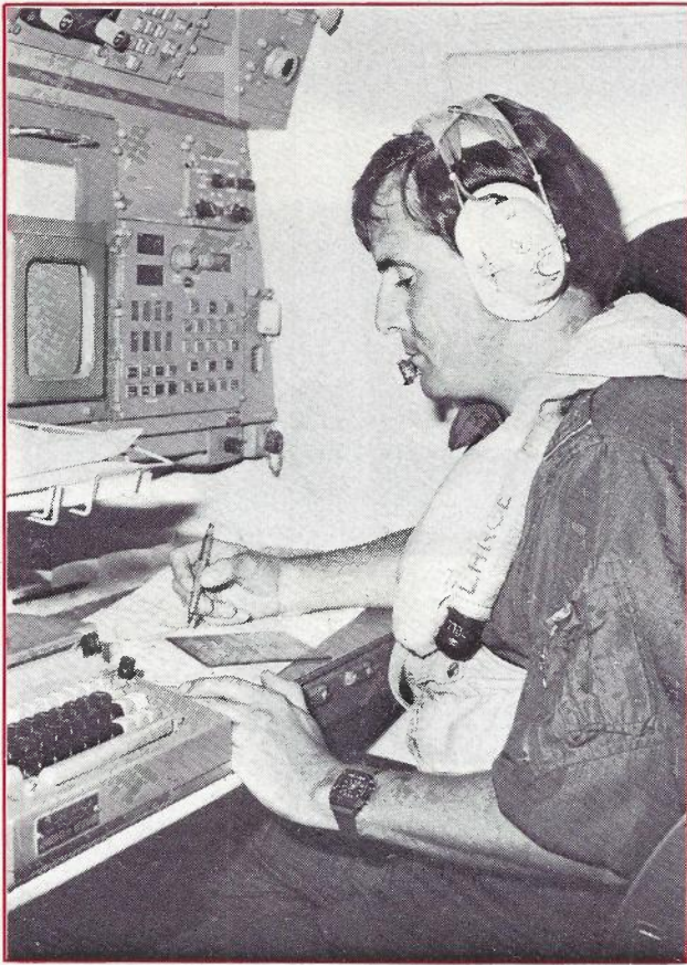
Fig. 4 — Partial view of the Navigator/radio operator position in a P3C maritime patrol aircraft. The operator is able to perform off-line electronic message preparation and editing before transmission.
