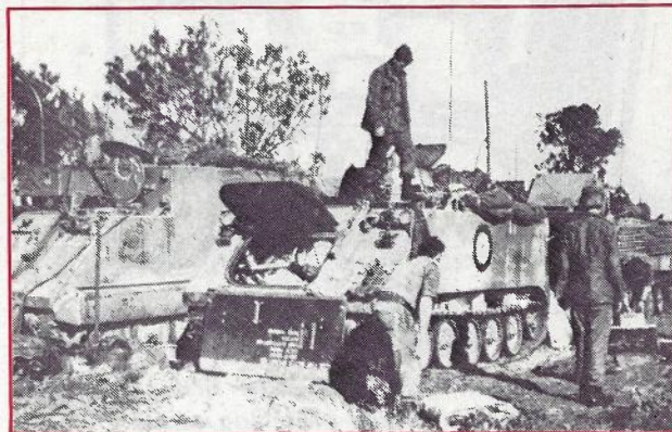
Fig. 7 — RAAF technical and operative personnel of ATTU checking out the communications equipment in a mobile air support facility which has been installed in a converted armoured personnel carrier.
