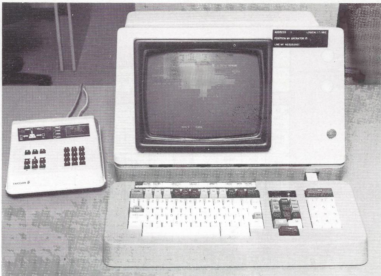
Fig. 7 — A SULTAN/LEOPARD Operator Position. Shown are the ACD Console and the SULTAN/LEOPARD VDU and keyboard.
