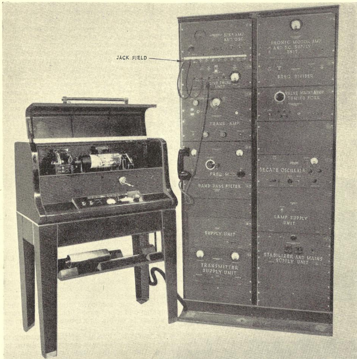
Fig. 7.—Transmitting Rack and Console.
