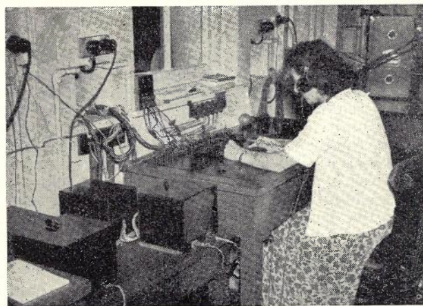
Fig. 11.—View of test equipment showing capacity unbalance set.
