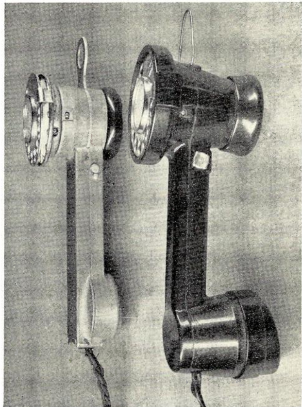
Fig. 2.—The new fabric filled phenol-formaldehyde body (compression moulded) and the old aluminium body (die cast).
