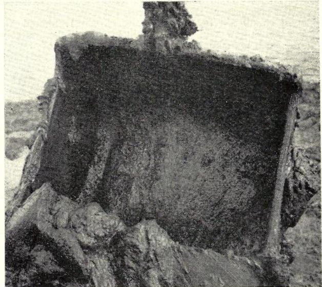
Fig. 2.—Drag-Line Excavator Bucket.
