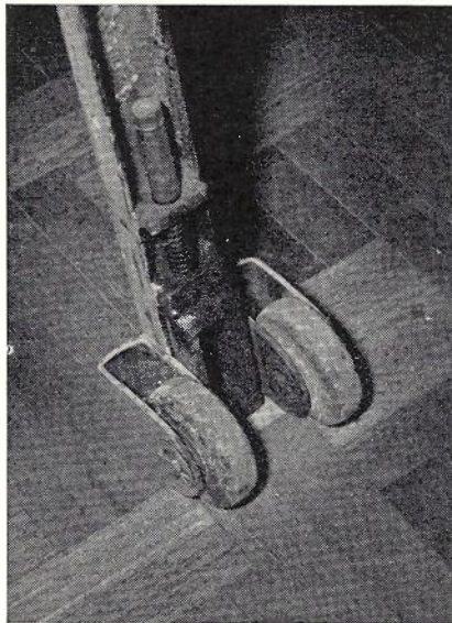
Fig. 18.—Lower end of channel iron showing lifting jack.
